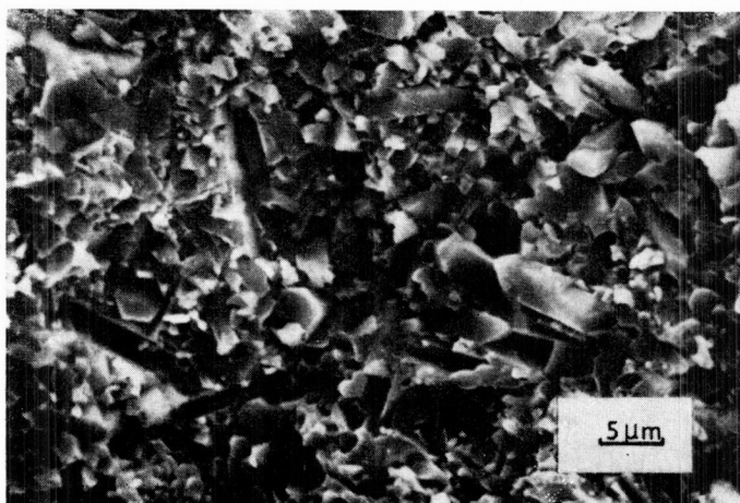
Fig. 12. Imprints of \beta -silicon nitride whiskers after their pulling out from the matrix.
