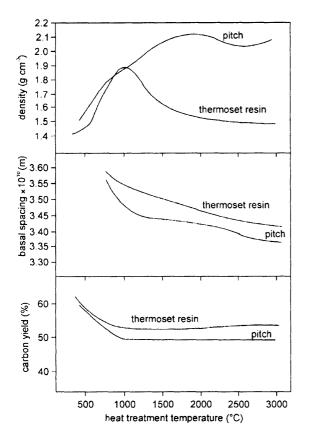
Figure 2. Characteristics of resin and pitch as a function of HTT [20].
