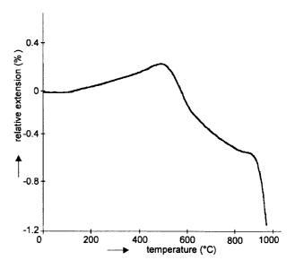
Figure 3. Dilatometric curve of the kaolin sample.
