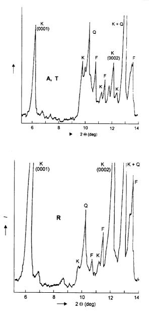
Figure 1. Diffraction patterns of the unfired samples for the axial, tangential, and radial directions. K - kaolinite, Q - quartz, F - feldspar.
