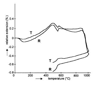
Figure 2. Dilatometric curves of the unfired samples measured in the tangential and radial direction.
