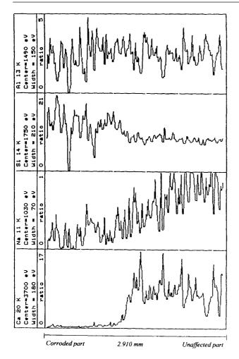
Figure 9. X-ray line analysis (EDS) of the specimen after 60 days of exposure to nitric acid at pH = 2 (magnification = 40×).
