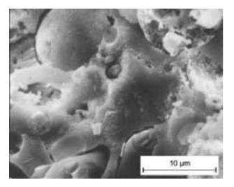
Figure 2. Microstructure of the corroded area at a region very close to the acid exposed surface of the specimen.
