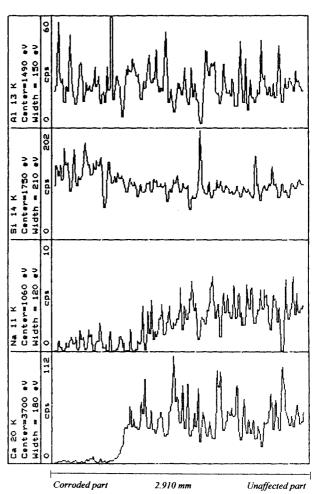
Figure 10. X-ray line analysis (EDS) of the specimen after 60 days of exposure to nitric acid at pH = 3 (magnification =  $100\times$ ).
