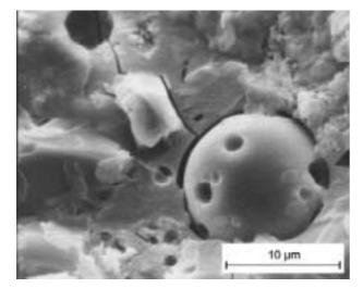
Figure 4. Unaffected microstructure of the specimen (uniform matrix along with an embedded fly ash particle).
