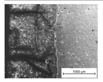
Figure 11. Corroded layer developed after 60 days exposure to pH = 2 nitric acid.
