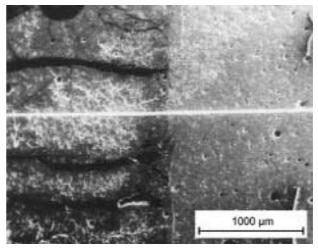
Figure 7. Corroded layer developed after 60 days exposure to pH = 1 nitric acid.
