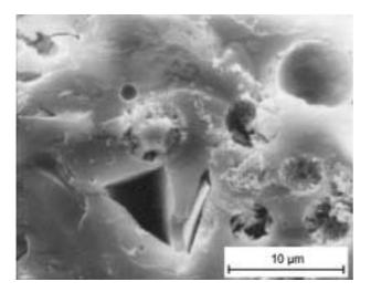
Figure 3. Microstructure of the corroded area somewhere in the middle of the corroded layer.
