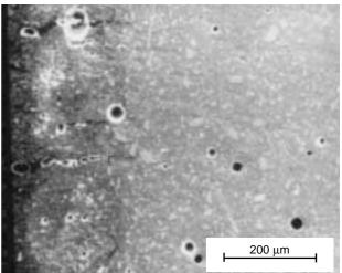
Figure 12. Corroded layer developed after 60 days exposure to pH = 3 nitric acid.
