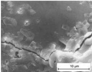
Figure 5. Unaffected microstructure of the specimen (uniform glassy matrix).
