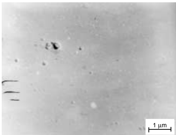
Figure 2. TEM micrograph of amorphous sample having composition 60V_2O_5.40B_2O_3 (mol.%) obtained by fast quenching.
