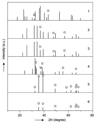
Figure 3. XRD patterns for the samples: Mg-I (1), Zn-I (2), Zn-II (3), Cd-I (4) heated to 900 °C, Cu-I (5), Cu-II (6) heated to 550 °C. All peaks are characteristic of corresponding orthosilicates (forsterite, willemite and  $Cd_2SiO_4$  respectively) except those indicated that are characteristic of accompanying crystalline phases: oxides (circles), tricadmium silicate (down triangles), enstatite (up triangles).
