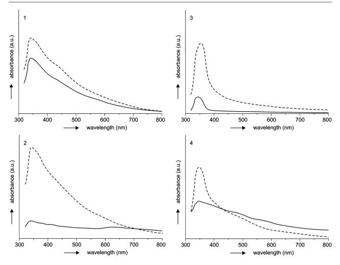
Figure 5. UV-VIS spectra for the samples: Cu-I (1), Cu-II (2), Zn-I (3) and Zn-II (4). 1, 2 ---- Si/Cu = 0, Si/Cu = 0.5; 3, 4 ---- Si/Zn = 0, Si/Zn = 0.5;
