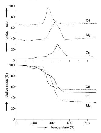
Figure 2. DTA and TGA curves for Mg-1, Zn-1 and Cd-1 dry gels, 5  $^{\circ}$ C/min.
