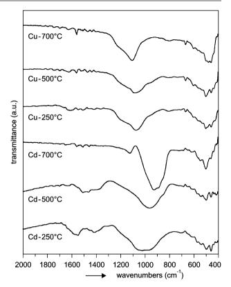
Figure 4. Thermal evolution at 250 - 700 °C of FTIR spectra for the samples Cd-I and Cu-I.
