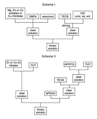
Figure 1. Flow-charts for the two preparation procedures.
