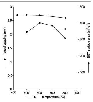
Figure 3. Basal spacing and BET surface area of aluminapillared micas heated at different temperatures. Solution loading was 24 mmol Al/g mica.
