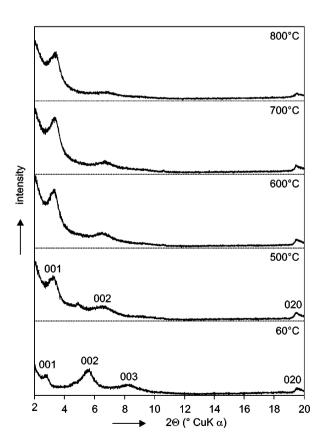
Figure 2. X-ray powder diffraction patterns of alumina-pillared micas heated at different temperatures. Solution loading was 24 mmol Al/g mica.
