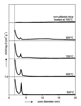
Figure 4. Pore size distribution curves of alumina-pillared micas heated at different temperatures. Solution loading was 24 mmol Al/g mica.
