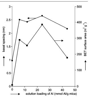
Figure 1. Basal spacing and BET surface area of aluminapillared micas heated at 700 °C plotted against solution loading per 1 g of host crystals.
