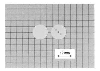
Figure 5. Photograph showing machinability of the sintered body of the alumina-pillared micas.
