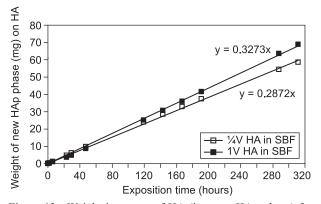
Figure 12. Weight increases of HA (i.e. new HAp phase) for partial ( $\frac{1}{4}$ V HA) and complete (1V HA) filling of the testing cell.
