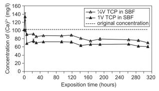
Figure 4. Concentration of calcium ions in the SBF solution for partial ( $\frac{1}{V}$  TCP) and complete (1V TCP) filling of the testing cells.
