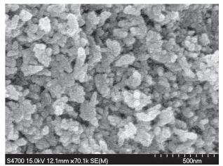
Figure 9. Surface of the material 1V HA (completely filled testing cell) after the exposure to SBF.
