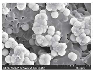
Figure 2. Surface of the material  $\frac{1}{4}$ V TCP (partly filled testing cell) after the exposure to SBF with the newly formed HAp phase.
