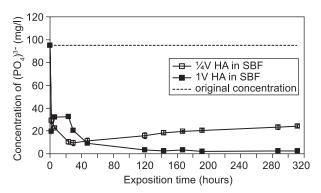
Figure 11. Concentrations of phosphate ions in the SBF solution in the partially ( $\frac{1}{4}$ V HA) and completely (1V HA) filled testing cells.
