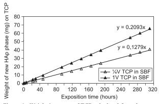
Figure 6. Weight increases of TCP calculated from decreases of concentration of  $(PO_4)^{3-}$  ions for partial (<sup>1</sup>/<sub>4</sub>V TCP) and complete (1V TCP) filling of the testing cells.
