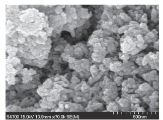
Figure 8. Surface of the <sup>1</sup>/<sub>4</sub>V HA material (from the partly filled testing cell) following the exposure to SBF.
