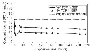
Figure 5. Concentrations of phosphate ions in the SBF solution for partial ( $\frac{1}{4}$ V TCP) and complete (1V TCP) filling of the testing cells.
