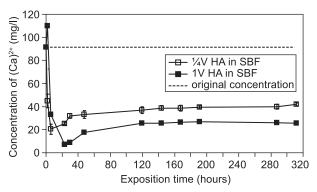
Figure 10. Concentrations of calcium ions in the SBF solution in the partially ( $\frac{1}{4}$ V HA) and completely (1V HA) filled testing cells.
