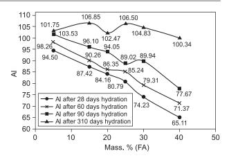
Figure 4. The activation index relative to fly ash replacement addition and hydration time (after 28, 90, and 310 days of hydration).
