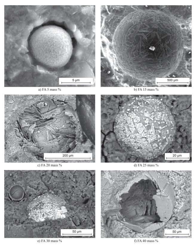
Figure 7. SEM images of mortar samples with replacement addition of FA (mass %) after 310 days of hydration.
