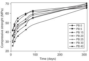
Figure 3. Development of compressive strength in mortars with fly ash replacement addition (0-40 mass %) relative to hydration duration (7-310 days of hydration).
