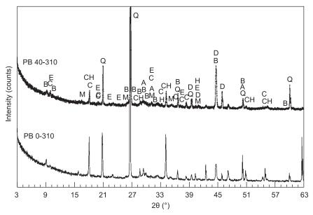
Figure 8. Comparison diffraction pattern for reference mortar (PB0) and mortar PB40 with higher part of fly ash (replacement addition fly ash is 40 mass%) after 310 days of hydration (Q - Quartz, M - Mullite, H - Hematite, CH - portlandite).
