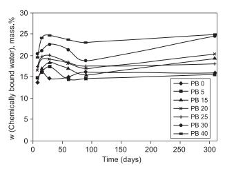
Figure 6. Change in the content of chemically bound water in mortar samples without and with FA replacement addition (5-40 mass %) relative to hydration time (7-310 days of hydration).
