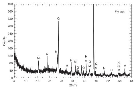
Figure 1. XRD powder pattern of the fly ash (Q - Quartz, M - Mullite, H - Hematite).
