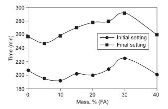
Figure 2. Effect of mass % of fly ash on the initial and final setting.
