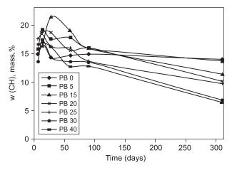
Figure 5. Change in the portlandite content in mortar samples without and with FA replacement addition (5-40 mass %) relative to hydration time (7-310 days of hydration).
