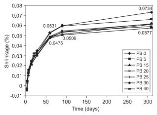
Figure 9. Drying shrinking of mortars containing fly ash replacement addition in the quantity from 0-40 mass %.
