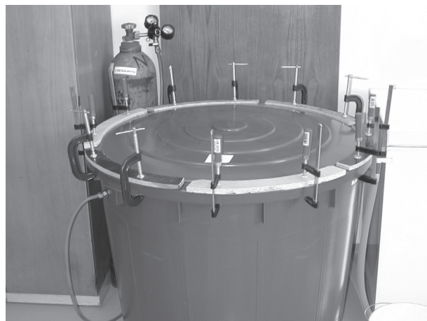
Figure 1. Complete pressurized tank with an atmosphere of 98% CO 2 .
