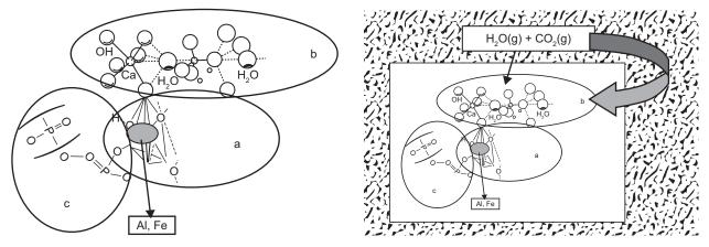
Figure 1. Formed cross-links (region a in part I, left) in the functional interfaces (entire part I, left) and the adverse influence of moisture (part II, right)
