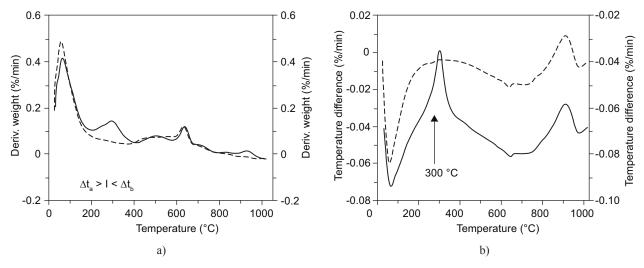
Figure 2. Typical DTG (a) and DTA (b) curves of MDF probes [8, 9, 11]; full lines with the events in the region from 200 to  $300^{\circ}$ C –  $\Delta t_b$  (DTG) and exoeffect at  $300^{\circ}$ C (DTA), denoting the occurrence of Al(Fe)–O–P cross-links (synthesis successful), dashed lines – no events in the region from 200 to  $300^{\circ}$ C due to the absence cross-links (synthesis not successful).
