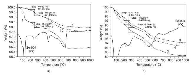
Figure 4. The evaluation of mass losses on TG curves in the temperature region  $200-300^{\circ}$ C which is sensitive on the presence (and thermal decomposition) of Al(Fe)–O–P cross-links; a) raw mixes mechanochemically treated for the duration of 5 minutes (in Table 3 referred as A. M., 5 min), b) final MDF probes [8, 9, 11] (in Table 3 referred as F. P.).
