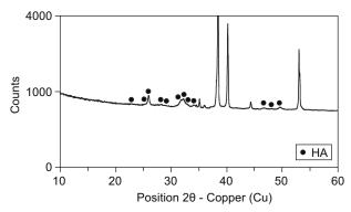
Figure 7. XRD difraction pattern for the coating SAN after in vitro test.
