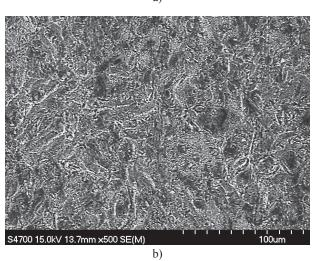
Figure 1. (SEM) Surface of titanium substrate after: a) grinding, b) leaching in HCl.
