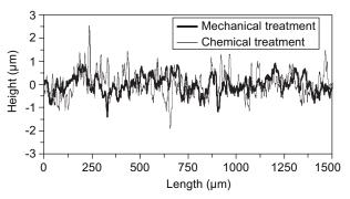
Figure 2. Profile comparison of Ti substrates after mechanical and chemical treatment.
