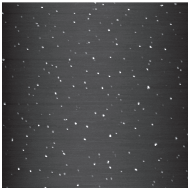
Figure 2. A micrograph of zirconia particle monolayer deposited on mica surface (AFM, semi-contact mode, scan size 5 \times 5 micrometers).
