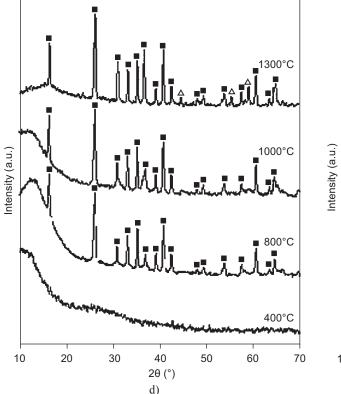
diffractograms of  $G_3$ ,  $G_4$  and  $G_5$  samples, apart from mullite,  $\alpha$ -Al<sub>2</sub>O<sub>3</sub> (JCPDS#46-1212) [28] reflections were observed and in  $G_5$  CoAl<sub>2</sub>O<sub>4</sub> (JCPDS# 44-0160) [29] phases are observed (Figure 1e).
