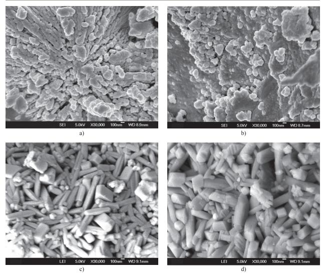
Figure 6. FESEM of mullite precursor gels doped with Cobalt sample G<sub>1</sub> and sample G<sub>5</sub> sintered at 1000°C and 1300°C.
