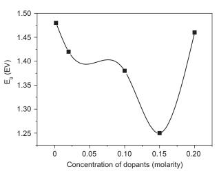
Figure 5. Activation energy  $(E_g)$  vs concentration curve of mullite precursor gels sintered at 400°C, 800°C, 1000°C and 1300°C containing increasing concentration of cobalt.
