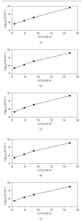
Figure 3. Resistivity  $(\log_{10} \rho)$  versus  $1/T \times 10^{-4}$  graph of mullite precursor gels sintered at 400°C, 800°C, 1000°C and 1300°C containing increasing concentration of cobalt.
