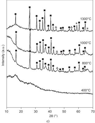
Figure 1. X-ray diffraction pattern of mullite precursor gels sintered at 400°C, 800°C, 1000°C and 1300°C containing increasing concentration of cobalt.
