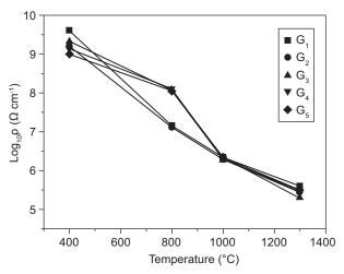
Figure 4. Resistivity versus Temperature (°C) of mullite precursor gels sintered at 400°C, 800°C, 1000°C and 1300°C containing increasing concentration of cobalt.
