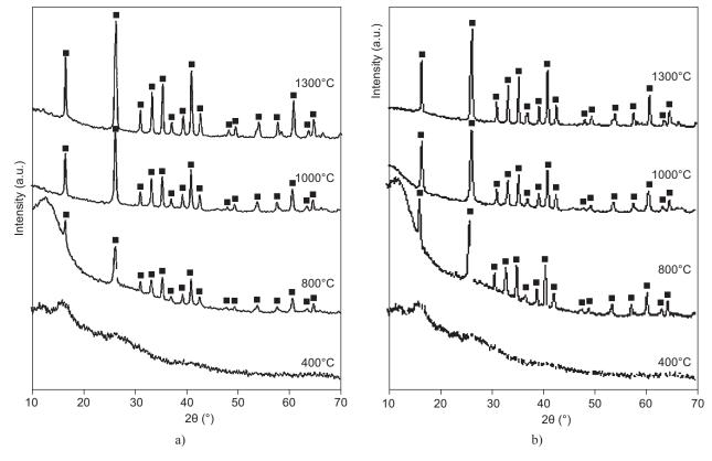
Figure 1. X-ray diffraction pattern of mullite precursor gels sintered at 400°C, 800°C, 1000°C and 1300°C containing increasing concentration of cobalt *(continue on next page)*.
