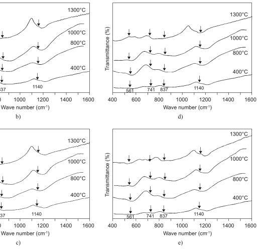
Figure 2. FTIR bands of mullite precursor gels sintered at 400°C, 800°C, 1000°C and 1300°C containing increasing concentration of cobalt.
