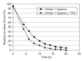
Figure 6. Variations of residue on 45  $\mu$ m sieve versus grinding time in ball mill.
