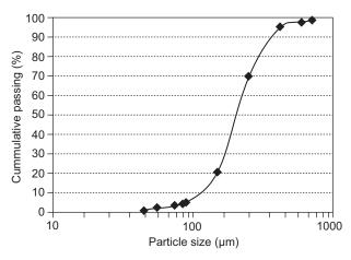
Figure 1. Particle size distribution of type II Portland cement clinker.
