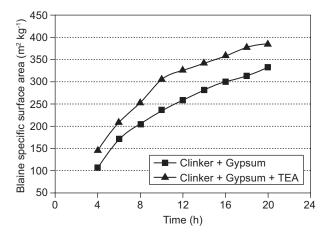
Figure 3. Variations of Blaine specific surface area versus grinding time in ball mill.
