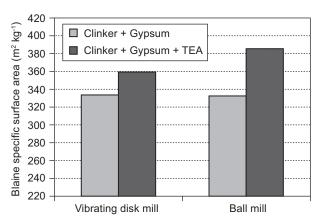
Figure 4. Effectiveness of TEA on Blaine specific surface area in ball and vibrating disk mills.
