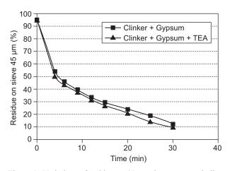
Figure 5. Variations of residue on 45  $\mu$ m sieve versus grinding time in vibrating disk mill.
