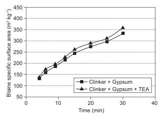
Figure 2. Variations of Blaine specific surface area versus grinding time in vibrating disk mill.
