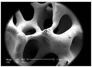
Figure 5. SEM photograph of alumina foam.
