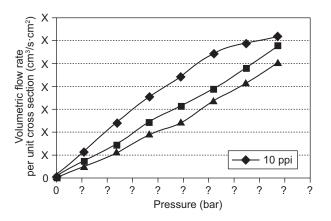
Figure 6. Volumetric flow rate of water per unit cross section of alumina foams with different pore densities.
