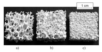
Figure 3. Morphology of alumina foams with pore density of a) 10, b) 17 and c) 27 ppi.
