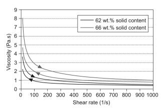
Figure 2. Viscosity curves of 62 wt. % and 66 wt. % solid content slurries.
