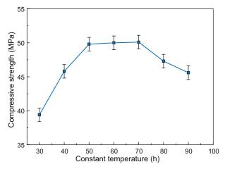
Figure 2. Effect of the constant temperature on the strength of the steam-cured concrete.
