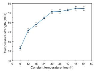
Figure 1. Effect of the constant temperature time on the strength of the steam-cured concrete.
