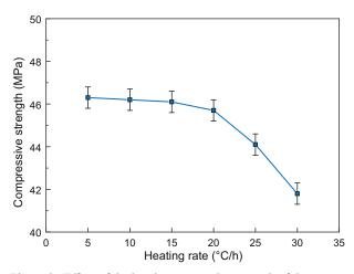
Figure 3. Effect of the heating rate on the strength of the steamcured concrete.
