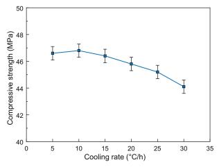
Figure 4. Effect of the cooling rate on the strength of the steam-cured concrete.
