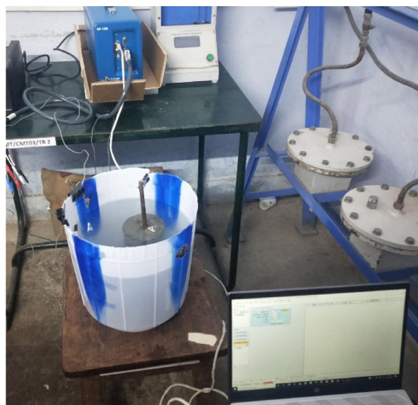
Figure 10. Corrosion evaluation – test set-up.
