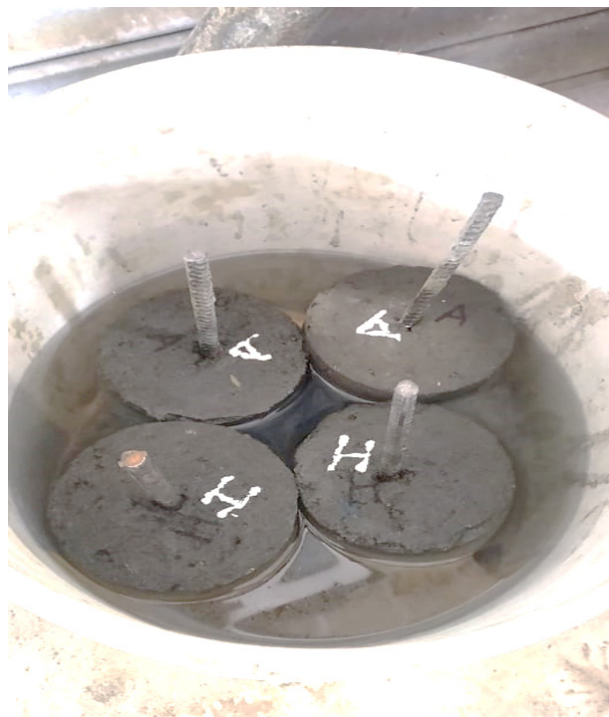
Figure 9. Test specimens in an NaCl solution.
