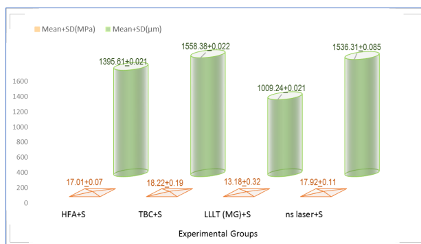
Figure 4. Mean and (SD) of the surface Ra and SBS in the NCC after applying different surfaces. A strong direct correlation exists between the Ra and the repair bond strength.
